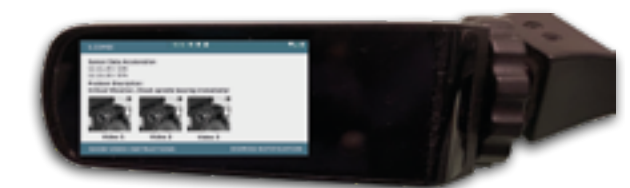
The alarm / event window opens automatically when a threshold value is exceeded.
